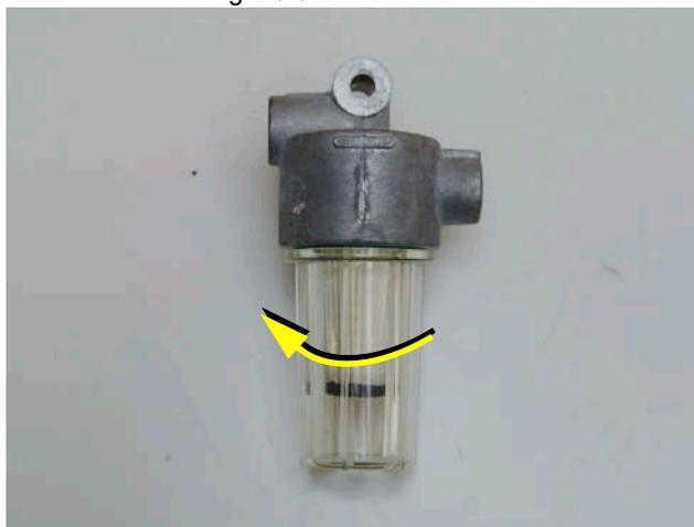
Unscrew the filter element from the mount (left hand rotation).
