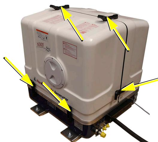
To open the lash closures pull the handle in arrow direction and lift the lash of the closure pin. After lifting off the lashes, the sound isolation cover upper part can be removed.
