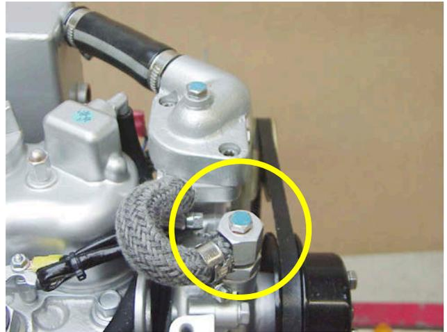
**Open de-aerating screw at the thermostat-housing**
