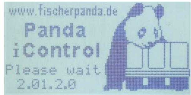
Fig. 13.3.1-2: Hardware version, generator type, and software version in default display
