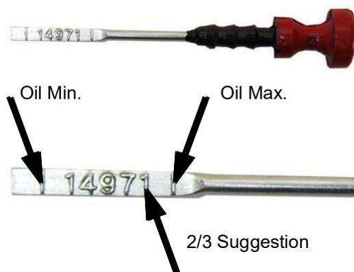
Oil should be refilled, if the oil-level is under 1/3 between the minimum and the maximum mark.
