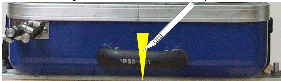
Fig. 8.4.5-2: Rubber hose for vent valve - example
