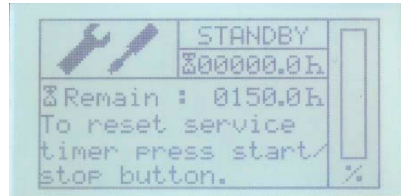
Fig. 15.4.7-1: Resetting the time until the next service
