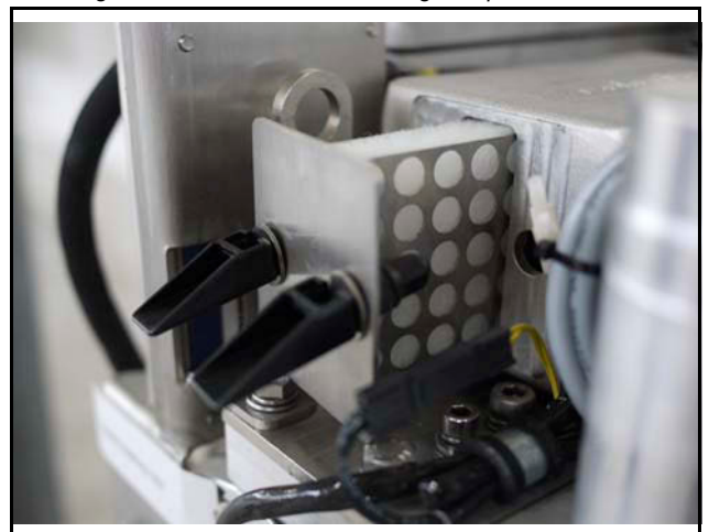
Fig. 10.10.2-3: Air suction housing with pull out holder
