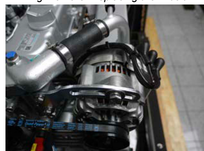
Fig. 10.10-3: Replacing the V-belt
