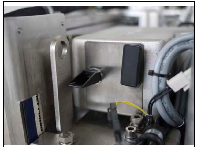
Fig. 10.10.2-2: Air suction housing with pull out holder
