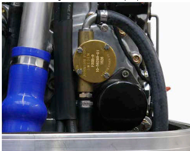
Fig. 8.12.3-2: Raw water pump
