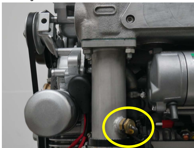
Fig. 6.3.6-2: Thermo-sensor at exhaust connection
