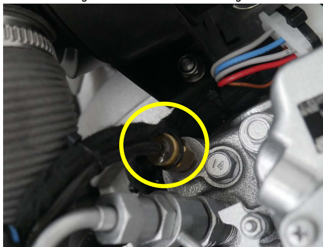
Fig. 6.3.6-1: Thermo-sensor at engine
