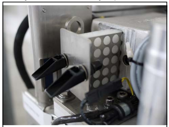
Fig. 9.10.2-3: Air suction housing with pull out holder
