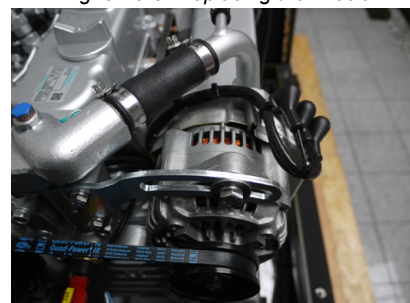
Fig. 9.10-3: Replacing the V-belt
