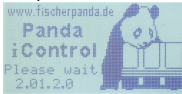
Fig. 14.3.1-2: Hardware version, generator type, and software version in default display
