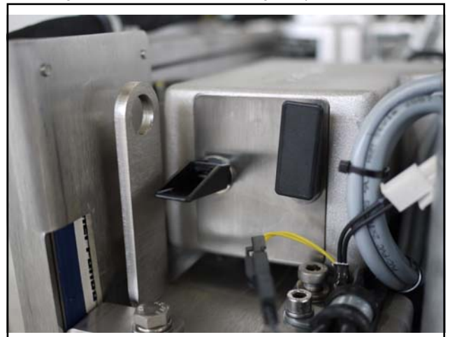
Fig. 9.10.2-3: Air suction housing with pull out holder
