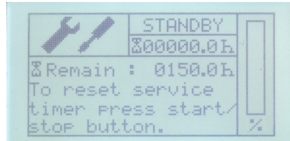
Fig. 14.4.7-1: Resetting the time until the next service
