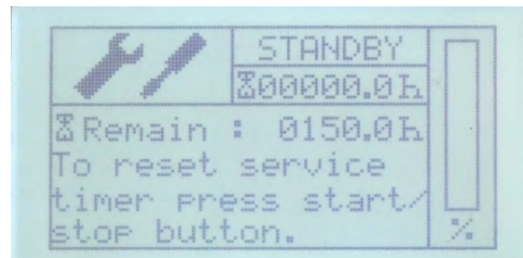
Fig. 15.4.7-1: Resetting the time until the next service
