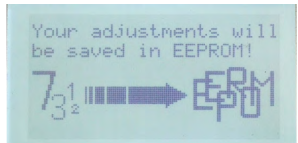
Fig. 15.4.5-1: Saving the values to the EEPROM
