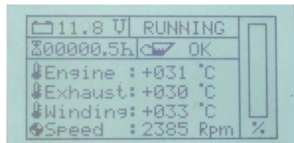
Fig. 15.3.3.4-1: Default display screen in operation mode
