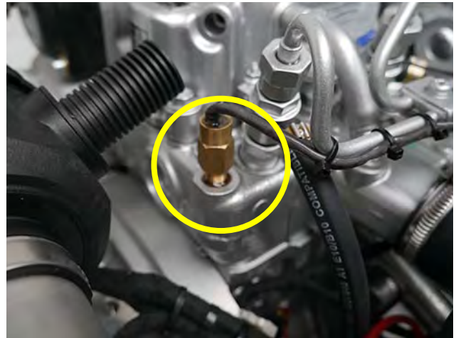
Fig. 7.2.6-1: Thermo.switch at engine
