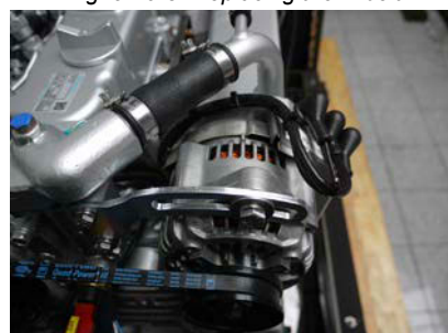
Fig. 9.10-3: Replacing the V-belt
