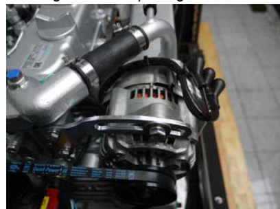
Fig. 8.10-3: Replacing the V-belt
