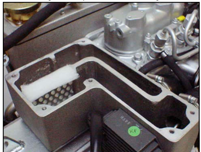
Fig. 8.10-2: Opened air suction housing
