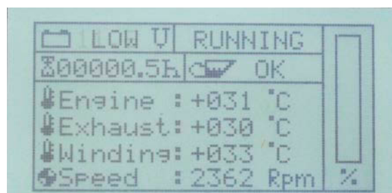
Fig. 16.1.1-1: Warning: „Battery power too low“
