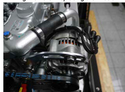
Fig. 10.10-3: Replacing the V-belt
