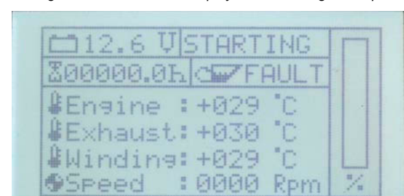
Fig. 13.3.3.2-2: Default display screen during start-up
