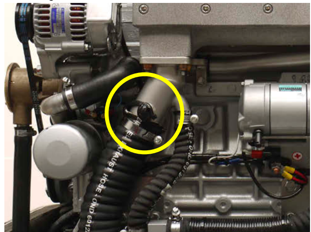
Fig. 5.3.6-2: Thermo-sensor at exhaust connection
