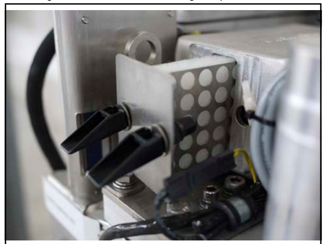
Fig. 8.10.2-3: Air suction housing with pull out holder
