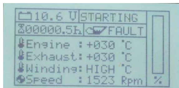
Fig. 16.1.1-2: Warning: „Winding temperature too high“
