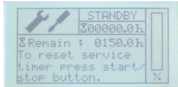
Fig. 13.4.7-1: Resetting the time until the next service
