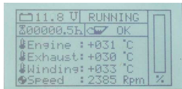
Fig. 13.3.3.4-1: Default display screen in operation mode
