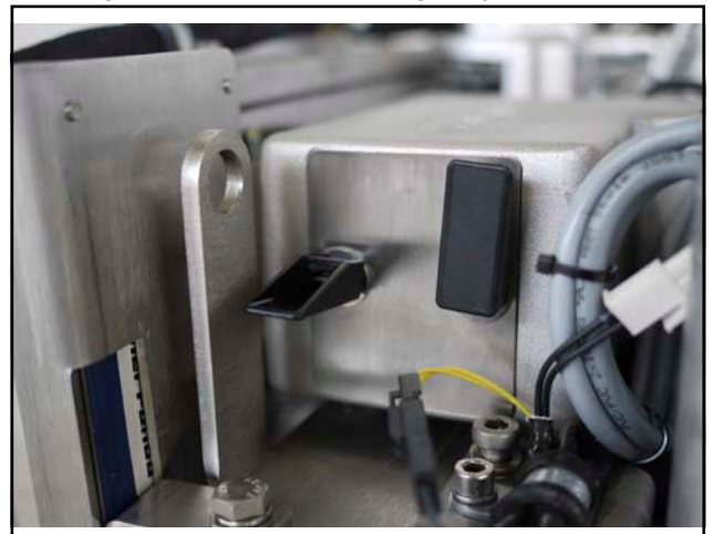
Fig. 8.10.2-3: Air suction housing with pull out holder
