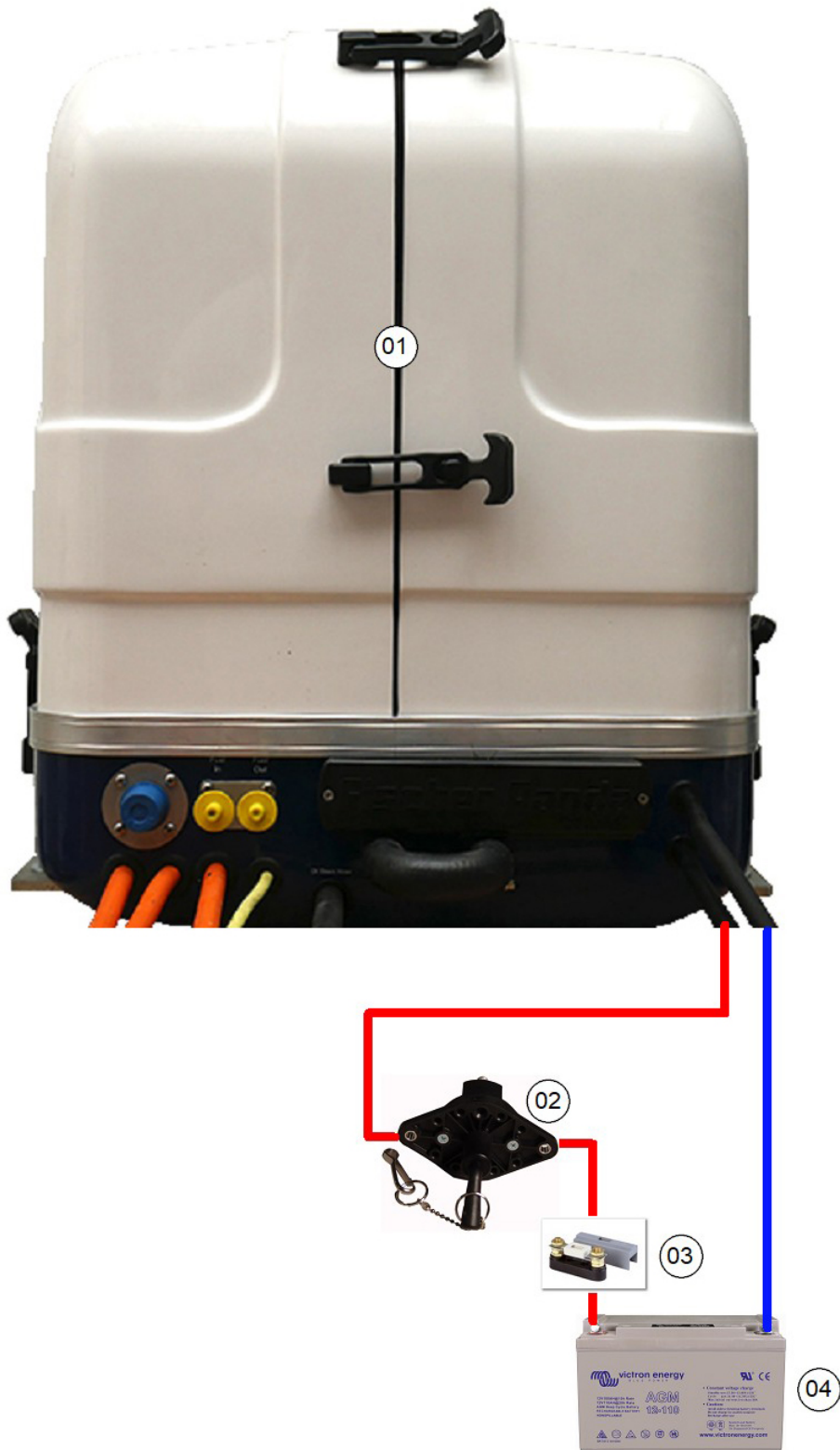
Fig. 7.9.3-1: 12 V starter battery connection - Schematic diagram
