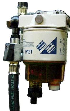
Fig. 10.7.1-1: Fuel filter with water separator
