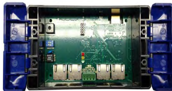
Fig. 12.1.4-1: fpControl CAN Interface - SAE J1939
