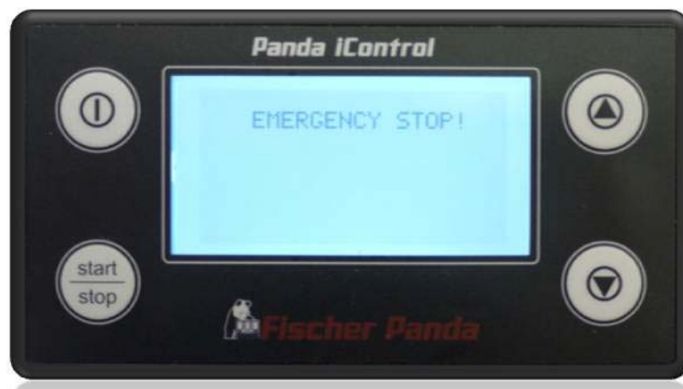
Fig. 12.5-2: Panel shows Emergency Stop
